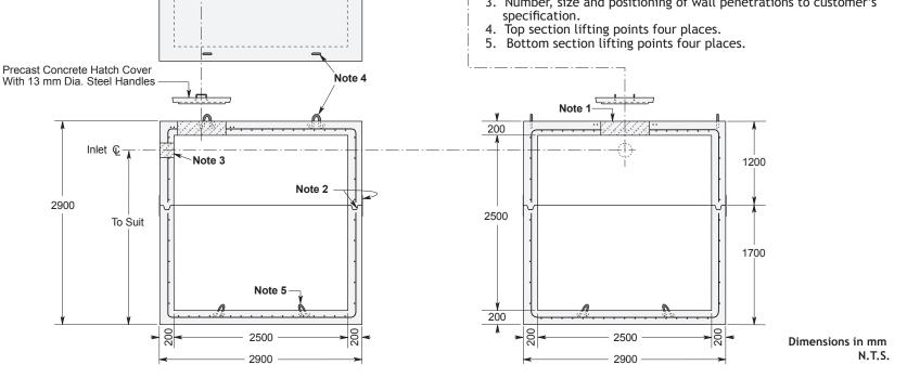
\* Commensurate with a 3 Metre burial over the top slab in firm soil and under an area of vehicular traffic.
