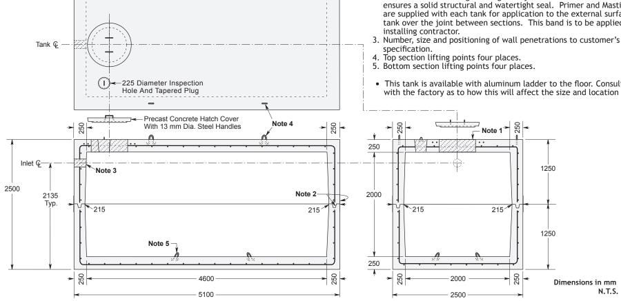
\* Commensurate with a 4 Metre burial over the top slab in firm soil. This tank is designed for burial in areas of vehicular traffic
