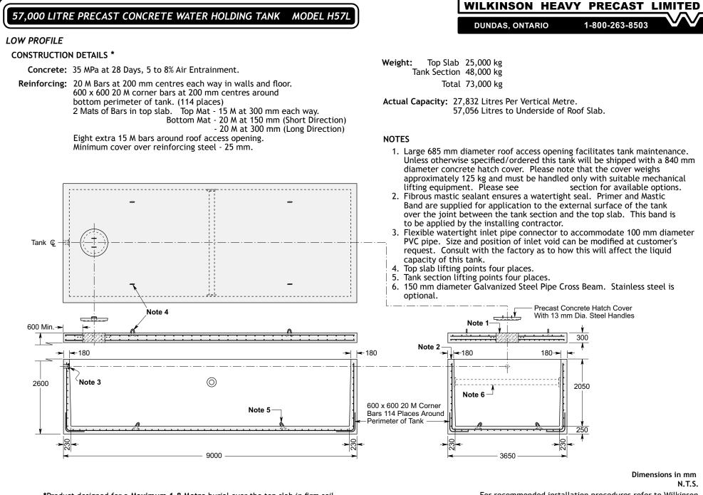
\*Product designed for a Maximum 1.8 Metre burial over the top slab in firm soil away from any area of vehicular traffic.
