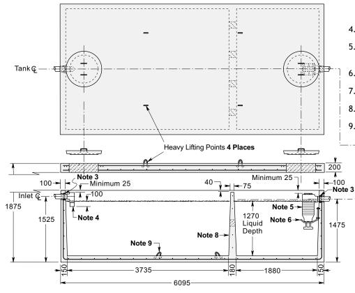
\*Product designed for a Maximum 1.2 Metre burial over the top slab in firm soil away from any area of vehicular traffic.
