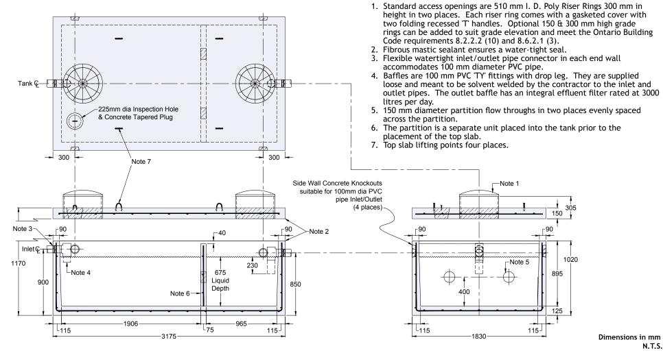
\*Product designed for a Maximum 1 Metre burial over the top slab in firm soil away from any area of vehicular traffic. For recommended installation procedures refer to Wilkinson \*\*NOTE: Since the liquid depth of this tank is less than 900mm it does not conform to CSA-B66.
