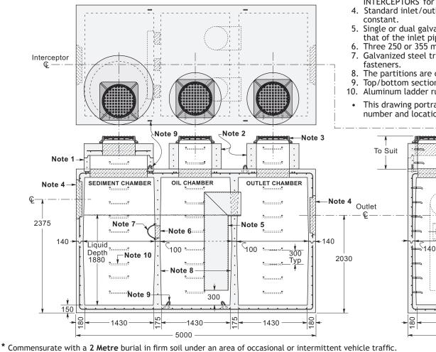
Total Internal Capacity: Wet & Dry Storage - 25 Cubic Metres
