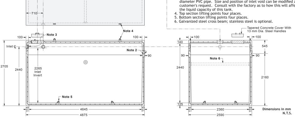
\* Commensurate with a 1 Metre burial over the top slab in firm soil away from any area of vehicular traffic.
