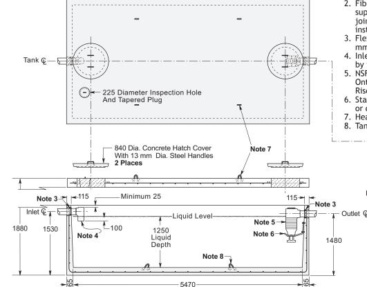
Actual Capacity: 15,068 Litres Per Vertical Metre. 22,602 Litres to Underside of Roof. 18,835 Litres to Invert of Outllet.
