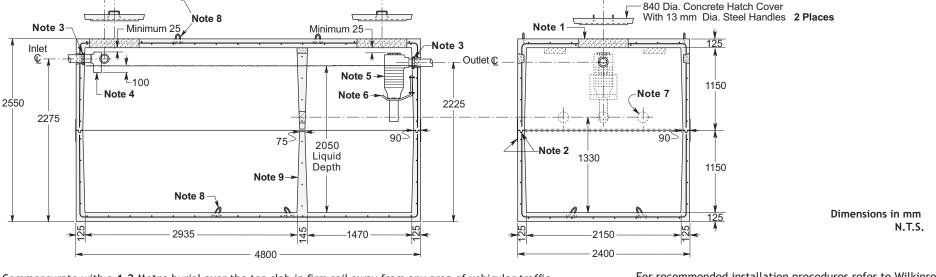
\* Commensurate with a 1.2 Metre burial over the top slab in firm soil away from any area of vehicular traffic.
