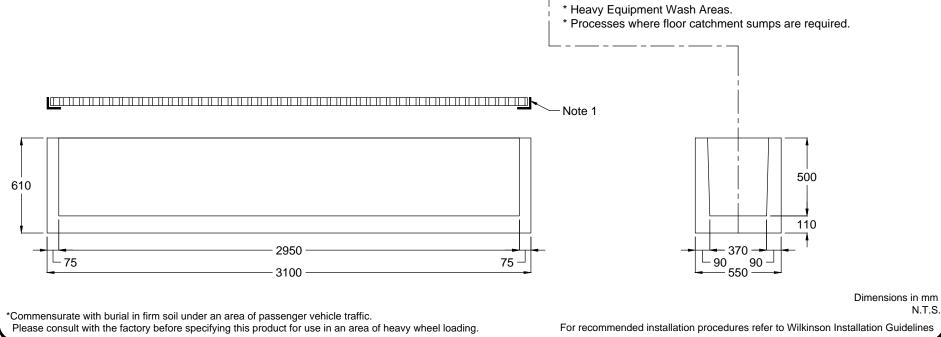
WARNING! IMPROPER INSTALLATION ESPECIALLY IN SATURATED SOILS CAN RESULT IN THE STRUCTURAL FAILURE OF THIS PRODUCT
