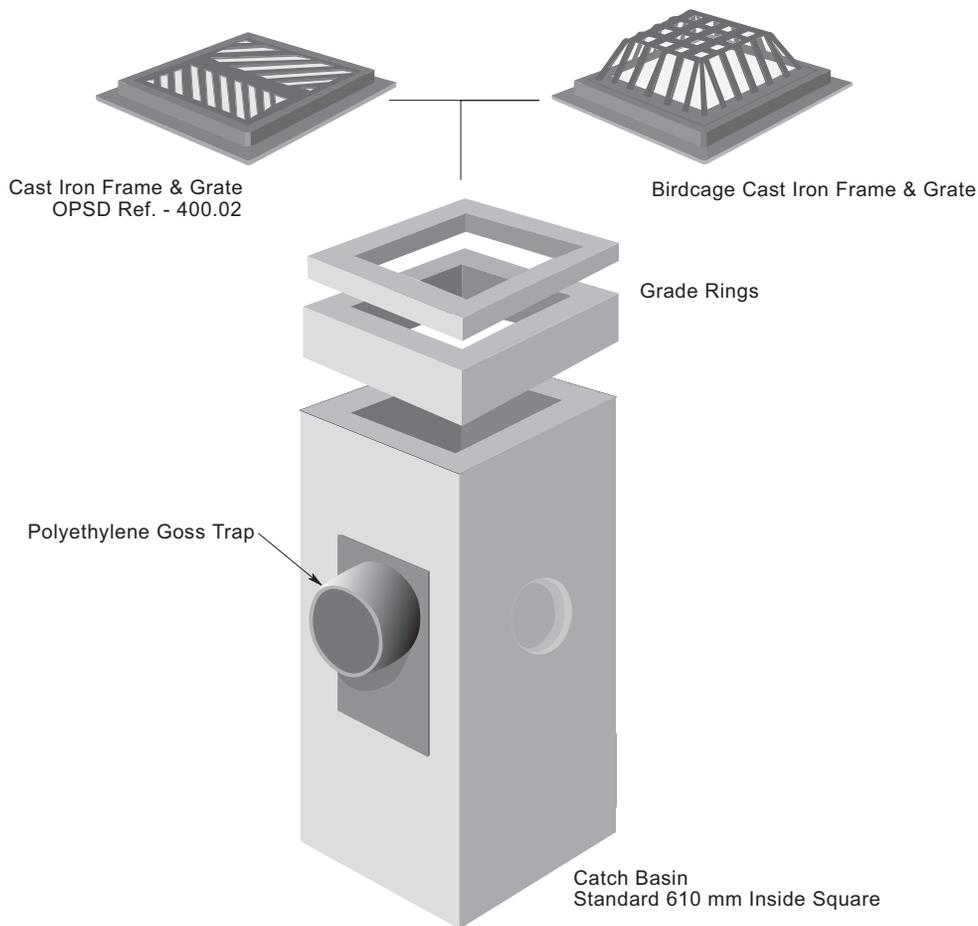
Cast Iron Frame and Grate and Birdcage Cast Iron Frame and Cover are available for 610 mm square and Double Catch Basins with or without Catch Basin Grade Rings.
