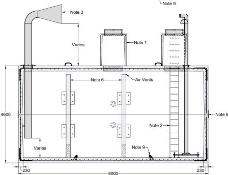
\*Product designed for a **Maximum 1.5 Metre** burial over the top slab in firm soil away from any area of vehicular traffic.
