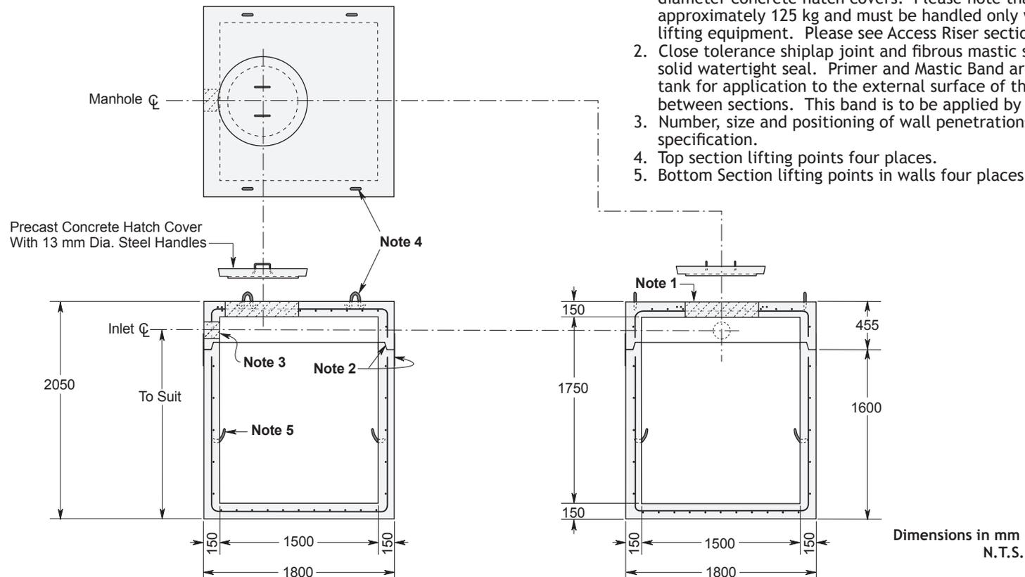
\* Commensurate with a 3 Metre burial over the top slab in firm soil and under an area of vehicular traffic.
