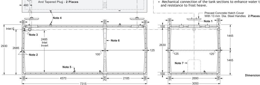
\* Commensurate with a 1.2 Metre burial over the top slab in firm soil away from any area of vehicular traffic.
