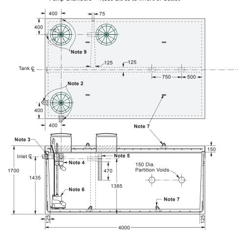
Weight: Top Slab 3760 kg Tank Section 9075 kg Total 12,705 kg
