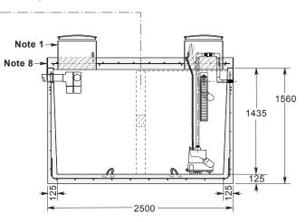
\* Commensurate with a 1 Metre burial over the top slab in firm soil away from any area of vehicular traffic.
