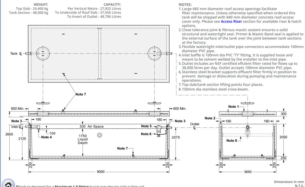
\*Product designed for a **Maximum 1.8 Metre** burial over the top slab in firm soil away from any area of vehicular traffic.
